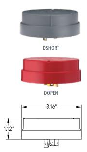
The CAP Series Shorting and Open caps are used with luminaires where lights are to be on continuously (shorting cap) or left off (open cap).
