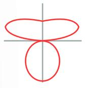
Proper offers a standard widespread indirect batwing and volumetric direct distribution to optimize balance of spatial luminance. Also, direct and indirect distributions can be controlled independently to facilitate the most effective and comfortable mix of illumination for any application need.
