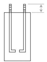
**NOTE:** STEEL POLES require 2 anchor nuts per bolt. Absolute minimum anchor bolt projection for .76" diameter bolts is 3.25". This is NOT the recommended projection. Consult Lithonia Lighting Technical Support.
